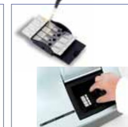
Pipette to test chips and start the GenomEra CDX assay run
